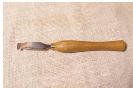
Bruce Everett's pieces: Salt and Pepper grinders. Ceramic Mechanism. Tool made to cut the internal groove of the mechanism
