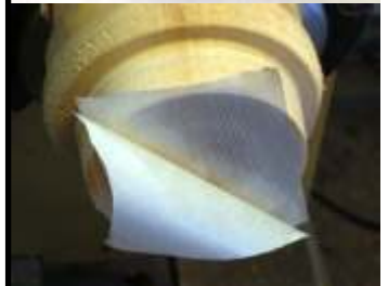
Double faced carpet tape chuck
