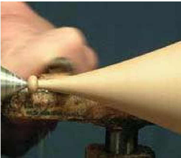
Photo 1: Use a spindle roughing gouge on its side to refine the shape of the finial.
