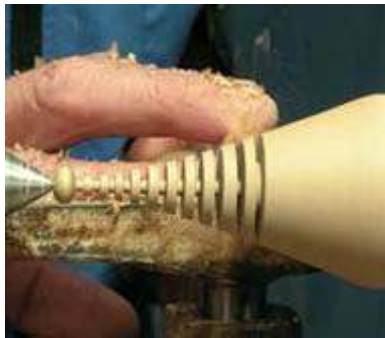
Photo 2: Cut the branch rings with a thin parting tool and leave a 1/8"-diameter tree trunk.
