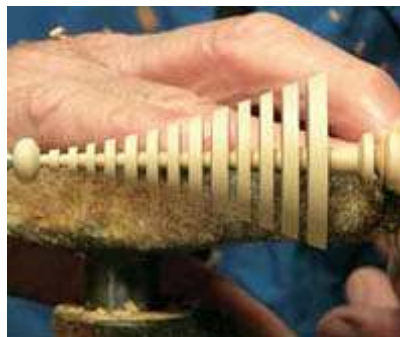
Photo 3: Create a stand for the tree and part the ornament from the chuck.
