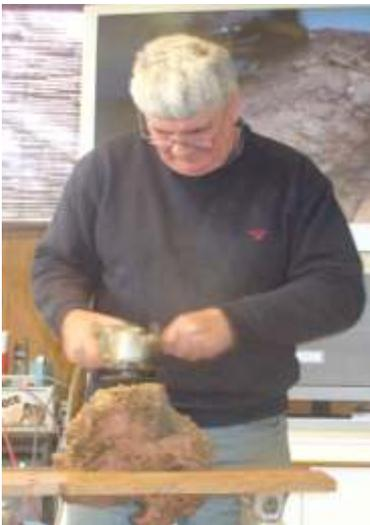
The use of sanders on angle grinders was also considered. Briefly use 60 or 80 grit for finer detail as finer grits will burnish the wood, but for polishing end grain 120 grit can be used successfully. The higher rpm is critical for good results as slower speeds will drag and cause tear outs.
