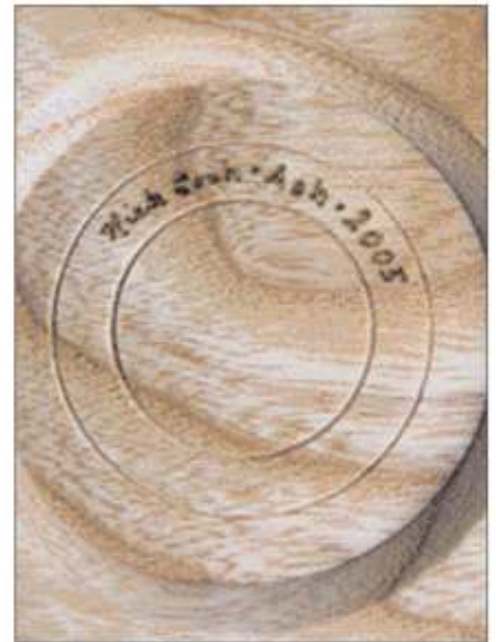
Two lines about 1/4" apart in the recess will provide you with an excellent place to sign your platter.
