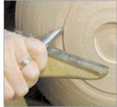
Use the tip of your bowl gouge to define the perimeter of the platter's foot. This photo shows detailing a chamfered foot.
