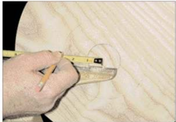
To mark off the foot of the plate, scribe a 5 1/2"- to 6"-diameter circle. The foot should be about one half the platter diameter.
