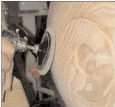
With the lathe running at about 500 rpm, begin power-sanding the platter bottom with a stiff 3"-diameter pad.
