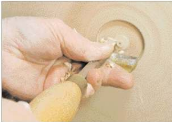
With a 3/8" bedan tool, cut the scroll-chuck recess. Many turners believe a slightly convex bottom has strong eye appeal.
