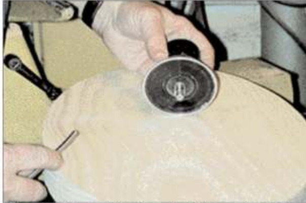
After cutting the round blank, mount a 1/2" screw chuck in the center. Check that the chuck fits snugly against the blank.
