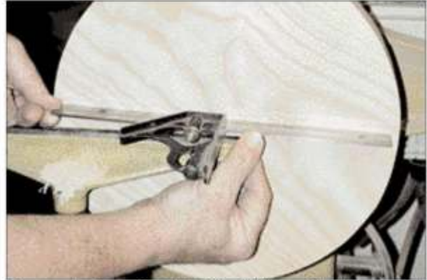
After turning the surface flat with a 3/8" deep-fluted bowl gouge, check for flatness with a 12" combination square.
