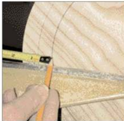
On the lathe, lay out a 1 1/2"-wide rim. This platter will have a crown centered about 3/4" from the platter's edge.
