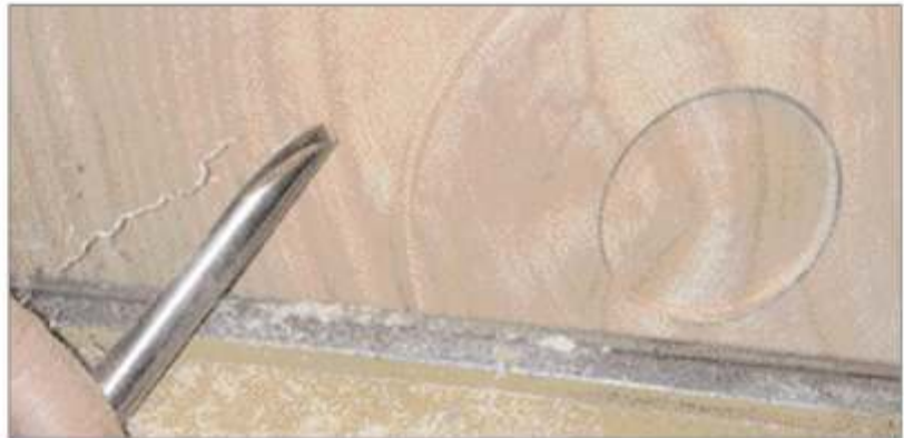
With your thigh as support, hold the bowl gouge nearly vertical to make finishing cuts. When you rest the heel of the bevel against the wood, you should see fine angel-hair shavings peeling off the platter.
