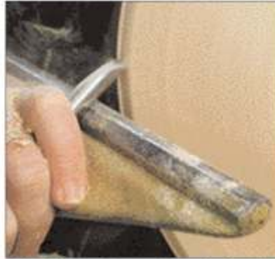
With a 3/8" bowl gouge, keep the handle perpendicular to the surface. The tool rest is positioned at 45 degrees.
