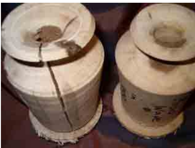
This picture shows the difference between two pieces that started out the same size and shape. The one on the right was microwave dried. Both from a walnut branch - a hard wood to dry without checking.
