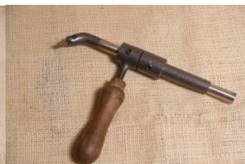
Jhon Crisp: New design in hollowing tool with side handle
