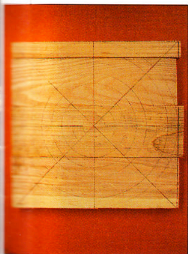
Photo 1 Four pieces of ash are glued together and marked out.
