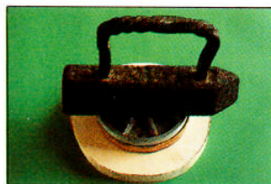
Photo 2 Fixing the blank to the scrap disc and faceplate.
