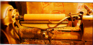
Photo 1 A cylinder of holly is turned to the correct diameter.
