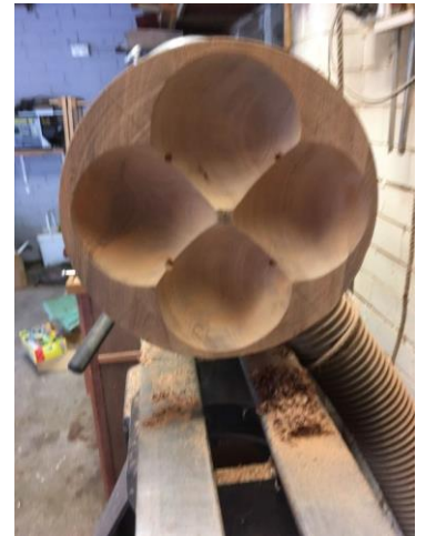
Four of the turnings cut to form scallops.
