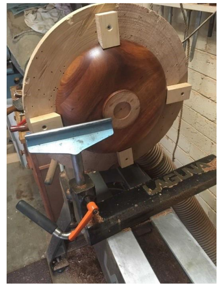
Bowl mounted on home made jig to remove the last chucking recess.
