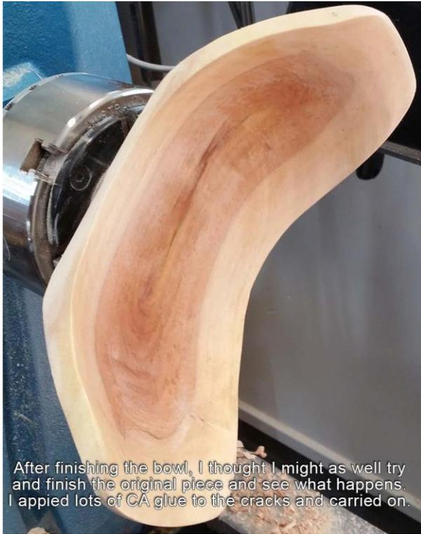
After finishing the bowl, I thought I might as well try and finish the original piece and see what happens. I applied lots of CA glue to the cracks and carried on.
