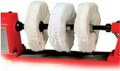
**MT.2 THREE STEP BUFFING SYSTEM:** A durable wax finish with MT.2 lathe-mounted polishing system. Buffing passes are made with a Tripoli buff (linen wheel), White Diamond buff (linen/flannel wheel), then Carnuba wax (flannel wheel).
