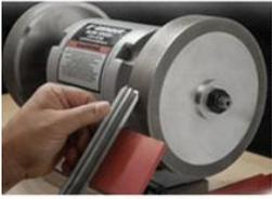
**CBN GRINDING WHEEL:** CBN is Cubic Boron Nitride. Don't have to worry about dressing or shaping like typical aluminum oxide wheels. It's perfect for sharpening HSS turning tools. You will achieve a super fine, sharp edge with polished bevel on either hardened tool steel or carbide. CBN Grinding Wheel are very quiet, produce very little sparks and generate very little heat when sharpening. The steel wheel body with hollow recessing bushing to make it light.
