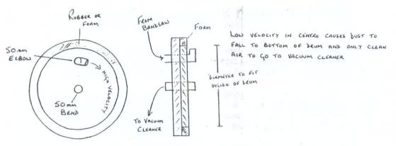
bottom compartment of the wheel) The dust collection point must be under the table for this system to work. If your saw has bottom guides (mine hasn't) you will need to cut the elbow or pipe carefully around the guides to minimise dust leakage. It, then, this causes the vacuum cleaner to complain through lack of air, a small opening must be provided elsewhere in the system, but not at the collection point.
