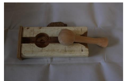
Ted Batty – Jig for cutting spoon blanks in half on a band saw
