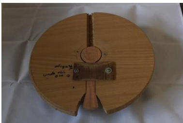
Ted Batty – Jig for holding spoon blanks on a lathe
