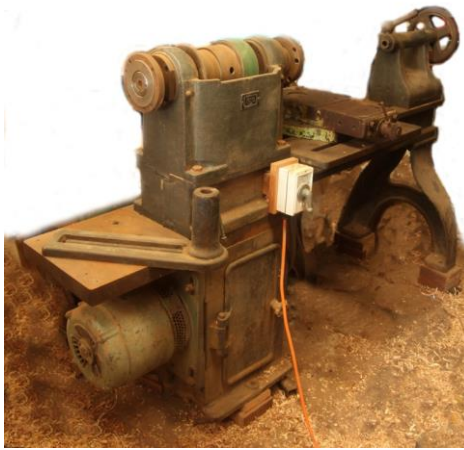
Demco ex metal-spinning lathe. Very heavy. Centre height 265 mm, capacity between centres 550 mm. Outboard turning facility. 3-phase motor. $1,000.
