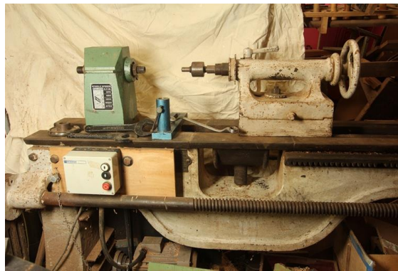
Long-bed lathe. Woodfast headstock on a Scottish Lang engineers flat bed. Has a carriage and a tailstock. Centre height 240 mm. capacity between centres 3.8. 3-phase motor easily replaceable. $1,000
