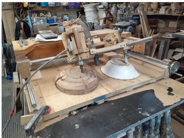
Carving & copying manual machine made by Gorgi Armen 920mm W. x 1230mm L. and unlimited length carving by moving the model
