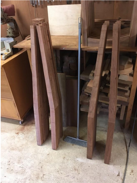
16 legs rough shaped off the Bandsaw
