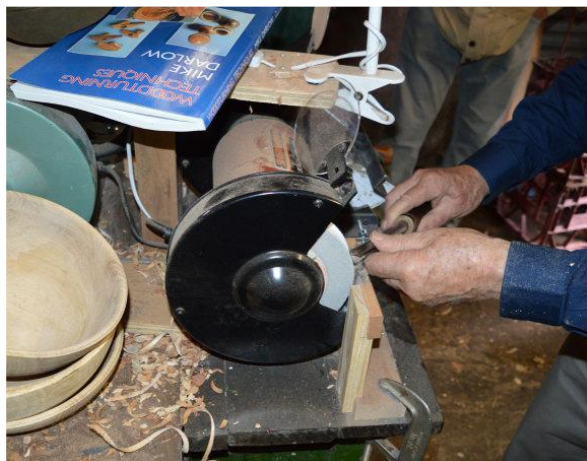
Sharpening a Bowl Gouge Darlow style
