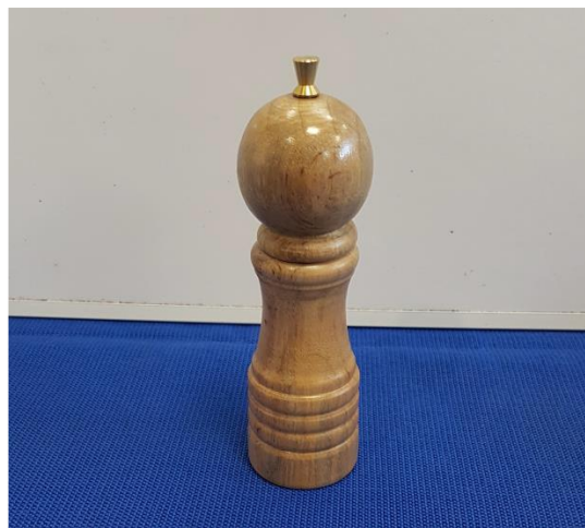
Lloyd Ross... a traditional shaped grinder made from old, dry 2003 Camphor Laurel. The finish is two coats of polyurethane. Lloyd, and others, commented on the difficulty of ensuring a concentric result.
