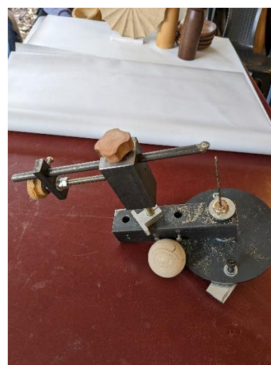
Catherine Ritter – homemade sphere cutter/jig.
