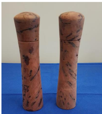
Jack Butler... a pair of Red Gum Burl Grinders. Glue and red oxide was used to infill imperfections and to stop the salt or pepper leaking from the walls of the grinders. Jack also commented on the importance of lathe alignment when turning grinders.
