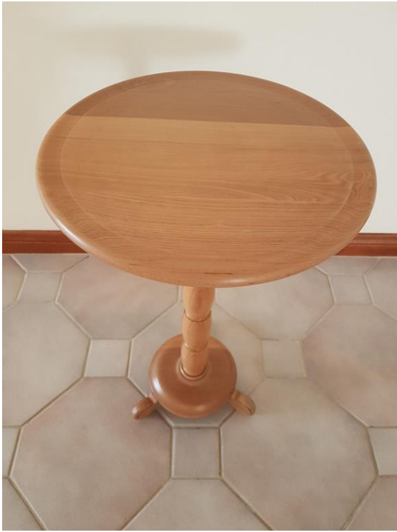
ROB LOVISA - BEDSIDE TABLE 600 High 380 Diameter. Used a recycled Coachwood benchtop - hence the different wood colours in the one piece. The Coach wood was nice to turn & once sanded to 600g it finished really well. Finish - Canuba Wax.
