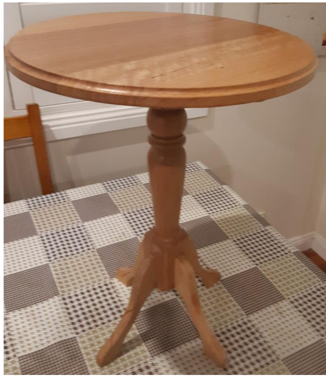
MICK BOUCHARD - SMALL SIDE TABLE made from Tasmanian Oak - Note ! All recycled timber. Finished in water based floor sealer. Polished with Bee's Wax.
