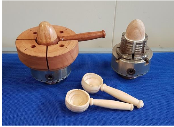
Also here, is a spoon jig, engineered by Jack with turned timber jaws that provide size adjustment flexibility. Another example is a split poly pipe chuck insert with cardboard packer for finishing turned eggs.
