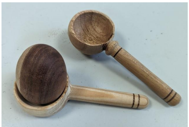
Alex Bendeli Alex described many ways to turn a perfect sphere using a sharpened cylinder and emphasised the benefits of working to a sketch or detailed drawing. The use of pre-cut accurate templates was also emphasised. The egg and spoon, turned from garden Viburnum exemplifies this! We have now seen it all... the use of a silicon toilet seal as a jam "chuck".
