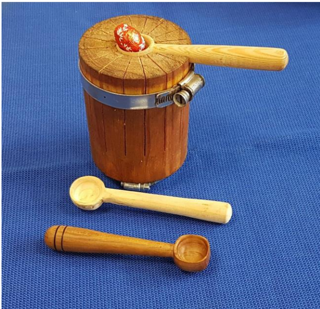
Tony Vidler. Another example of an adjustable jig for use with spoon turning accompanied by three salt spoons all turned from Pine.
