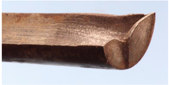
The tip of a traditional pattern long-hole-boring auger. These were manufactured in a range of diameters.
