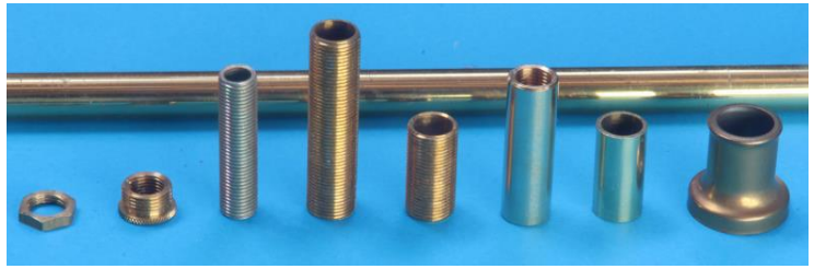
A selection of nipples etc is shown here in Figure 2. In Europe and Australasia these usually have 10 x 1 mm threads. A hand die or tap can be used to thread metal
