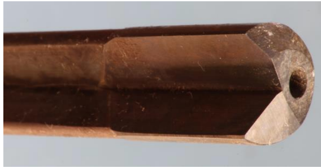
The tungsten carbide tip of a gun drill. Compressed air exits through the hole in the tip and blasts the chips back down the flute of the steel shaft. Gun drills are preferred if you're going to produce large numbers of lamps.
