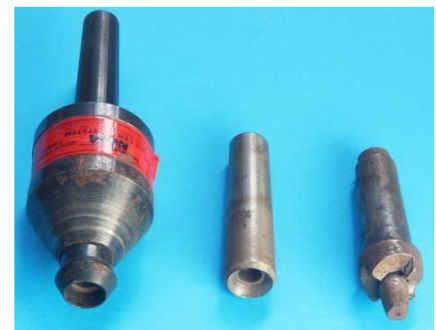
Figure 6: Centres for long-hole boring. Left, tail centre; a live hollow middle, a dead hollow tail centre; right a drive centre with an enlarged centre pin.
