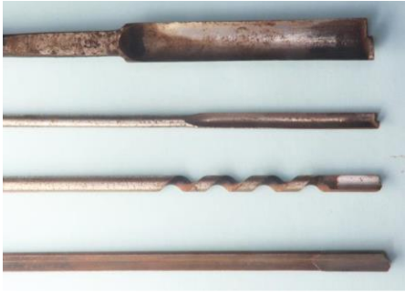
Three long-hole boring augers.
